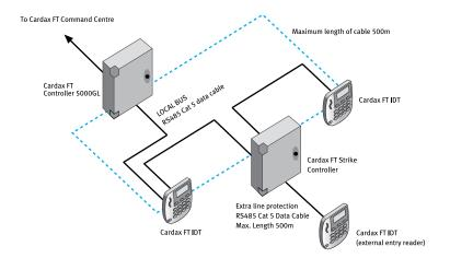
Cardax FT Intelligent Door Terminals connecting to a Cardax FT Controller 5000GL, with one reader on an external door connected to a Cardax FT Strike Controller for extra line protection.
